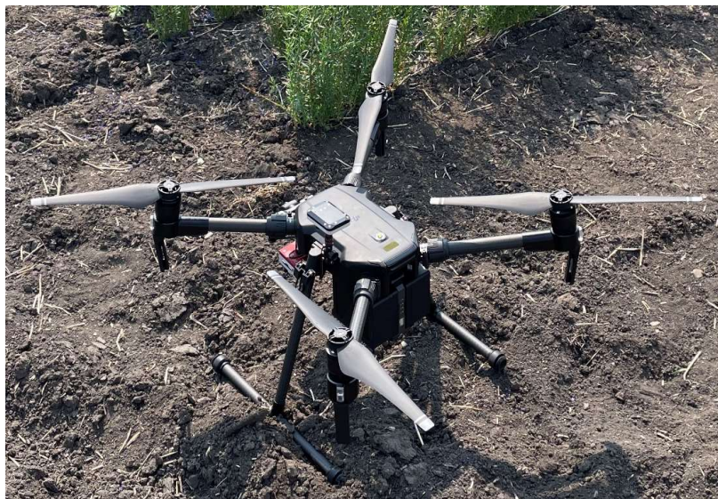
Drone – DJI M200 V2 with MicaSense Multispectral (RedEdge) camera
